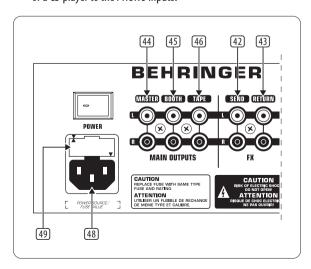
The DJX750 features an integrated effects loop for the connection of an external effects device. The MONITOR signal is taken at the SEND output
