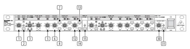
Fig. 2.3: Active control elements on the front panel of the SUPER-X PRO for stereo 2-way operation
