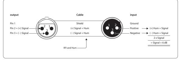
Fig. 4.11: Fig. 4.1: Compensation of interference with balanced connections
