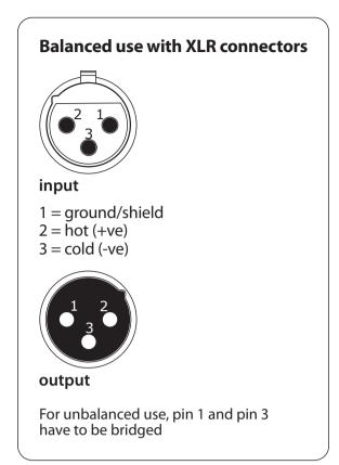
Fig. 4.12: Different plug types
