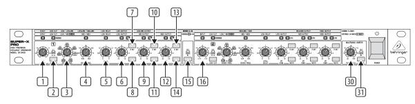
Fig. 2.6: Active control elements on the front panel of the SUPER-X PRO for stereo 3-way operation
