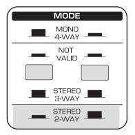
Fig. 2.2: Proper selection of the two MODE buttons for stereo 2-way operation
