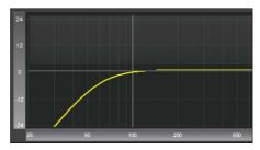
Illustration 5.2: Here the HiPass Output 2 Crossover is set to Linkwitz-Riley 24dB with the frequency set to 60.0Hz
