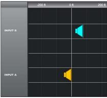
Illustration 5.1: Input B Delay is set to 75 feet. In this illustration, speaker array B is said to b 75 feet in front of Main speaker array A. The effect of air temperature is also automatically calculated for the total delay time using the Temperature value entered in the Setup Menu.
