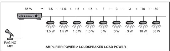
In fact working with 100V loudspeakers is rather simple, when done in the right way. Each 100V loudspeaker has a 100V transformer which can be set to a certain power, for example: 1,5 3 or 6W. As the example shows, the sum of all loudspeaker settings should never exceed the amplifier's power specifications.
