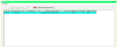
After launching the software, power the unit on and then connect it to the PC/laptop using a USB cable. Click on the "Search" button and any detected units will be displayed in the list. Clicking on a detected unit will open the EDID Commander window.
