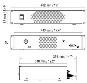
Do not obstruct the ventilation slots. Ensure adequate air flow around the iPS10.
