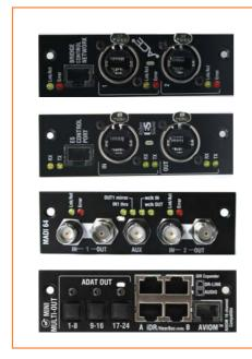
**ACE™** Adds a second ACE™ port. Use one socket for the link. Use the second socket for a redundant backup connection if required. Use a short cable to bridge the NETWORK over the ACE™ cable if needed.
