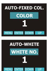
By setting all the units connected to the MASTER to DMX address 1, them will be synchronized with the Master unit following the chase selected on it, including TIME, WAIT, Pan&Tilt and Zoom position of the MASTER unit.
