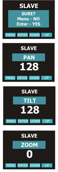
The SLAVE unit receive DMX signal from the MASTER unit. By setting all the SLAVE units connected to the MASTER, to DMX address 1, them will be synchronized with the Master unit following the chase selected on it, but running their own Pan&Tilt and Zoom position.
