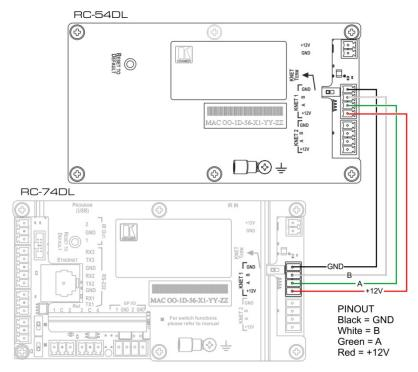
Figure 5: RC-54DL to RC-74DL Pinout Connection
