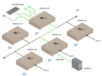
Figure 2.9 - Using USB devices under unicast mode.
