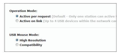
Under Active per request mode, multiple USB devices may be present on one or more Receiver units. However, only one Receiver unit can have USB control at a time.
