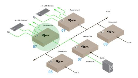
3. In order to assign USB control to a different Receiver unit, repeat steps 1 - 2
