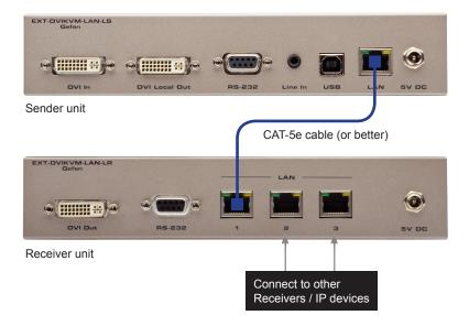
Although any LAN port on the Receiver unit can be used, using the LAN 1 port makes it easy to identify which Ethernet cable is used to connect the Sender and Receiver unit. LAN 2 and LAN 3 ports can then be used for connecting additional devices or when daisy-chaining Receiver units.
