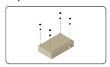
Step 4 Install countersink screws .
