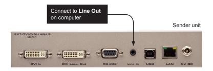
Note that any audio device (e.g. MP3 player, etc.) can also be connected to the **Line In** jack on the Sender unit.
