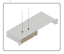
Step 6 Unit has been installed into rack tray.
