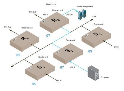
Figure 2.13 - Speaker connections in multicast mode.
