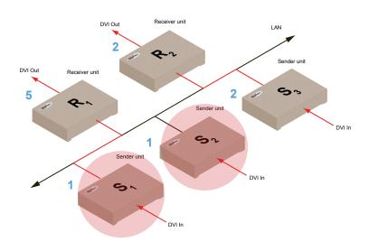
In order to solve the problem, in Figure 2.4, we would need to make sure that each of the Sender units is set to a unique channel number.
