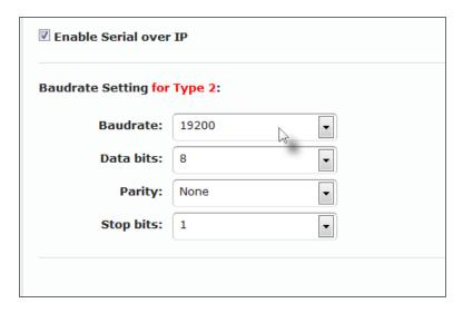
Make sure that the Enable Serial over IP box is checked.
