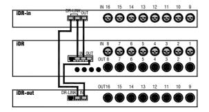
**Fully expanded iDR-8** This diagram shows the **iDR-8** with both the input and output expander fitted. Note the connection of DR-Link which is daisy chained from one unit to the next. If an **iDR-switch** unit is also fitted then daisy chain DR-Link from the last expander to the switch box. Make sure you plug into the correct DR-Link socket.
