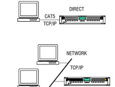
The **iDR-8** uses TCP/IP to communicate with a PC or distributed network via a CAT5 Ethernet link. It can also communicate over a dial-up connection using PPP via its RS232 port. The faster Ethernet connection is recommended for iDR configuration purposes. Note that the front panel RS232 port is intended for operating code update. The rear panel RS232 port is intended for remote interrogation of the unit via a modern.
