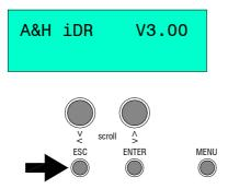
With the face plate removed, press and hold the ESC key to view the current version of operating code running in the unit.
