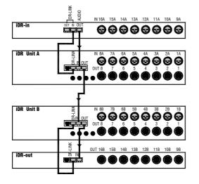
**Expanded multiple iDR-8 system** This diagram shows an iDR system with two **iDR-8** units and both expanders fitted. DR-Link is only required to connect to the expanders, not between the main units. Make sure you connect DR-Link to the **iDR-8** associated with each expander. Make sure you plug into the correct DR-Link socket. In this case do not daisy chain DR-Link from one expander to the other.
