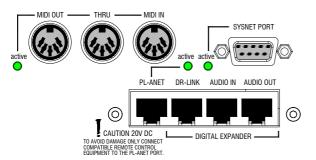
MIDI Three 5pin DIN connectors provide MIDI IN, THRU and OUT. These work with the popular MIDI interface standard. The MIDI channel number can be selected. Check the iDR System Manager Help file for more information on using MIDI with iDR. Refer to the Allen & Heath iDR MIDI Protocol document for details on how to control the parameters using MIDI messages. This can be downloaded from our web site. Use MIDI cables up to 15 metre (50 feet) in length.
