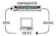
The way the **iDR-8** is set up and the contents of any patches which have been created is stored as a 'configuration'. It can be archived as a .cfg file on your PC. Any number of configurations can be named and stored. You can load a configuration back into the unit using the iDR System Manager. Refer to the section about Configurations and Patches later in this user guide and the iDR System Manager Help file for more details.
