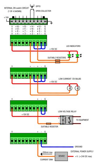
**Using the logic outputs** Each output is optocoupled to isolate the **iDR-switch** from the connected equipment. It provides an open collector output with floating collector (+pin) and emitter (-pin).
