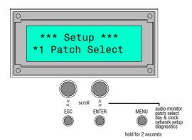
Before your PC can take control of the iDR-8 you need to set up its unit name and communication settings. This is done using a simple front panel menu system. Once communication is established between the PC and iDR-8 you use the iDR System Manager software to configure and control the unit.
