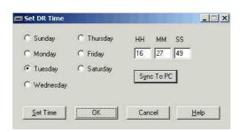
Before starting to configure the unit, check that the time and day of week are correctly set. Depending on the current LCD settings these may or may not be displayed. There are two ways to change the settings:
