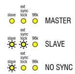
**Master** / **Slave** When **iDR-8** units are linked one becomes the master and the others the slaves. This is so that they synchronise their audio communication. The first **iDR-8** in the chain automatically becomes the master. However, this is not the case in a 'loop back' system where the audio from the last unit is linked back into the first unit. Here, you need to force one unit to become the master. This is described later.
