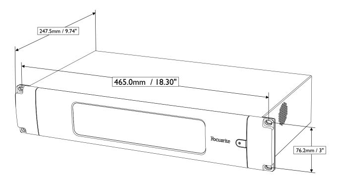
RedNet 3 requires 2U of vertical rackspace and at least 350 mm of rack depth, to allow for cables. RedNet 3 weighs 4.34 kg, and for installations in a fixed environment (e.g., a studio), the front panel mounting screws will provide adequate support. If the units are to be used in a mobile situation (e.g., flight-cased for touring, etc.), consideration should be given to using side support rails within the rack.
