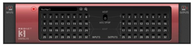
**Port activity**: Each of the RedNet 3's 32 inputs and 32 outputs has a virtual LED which illuminates to confirm the presence of an audio signal on that channel. Note that as the maximum number of channels is reduced at higher sample rates, the number of LEDs which may appear active is dependent on the sample rate.
