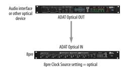
Figure 4-6: Two setups for synchronizing an optical device with the 8pre.
