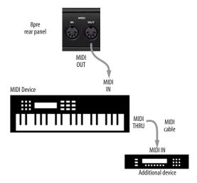
${\it Figure 4-3: Connecting \ additional \ devices \ with \ MIDITHRU \ ports.}$
