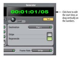
Figure 12-2: Setting the time code start time.
