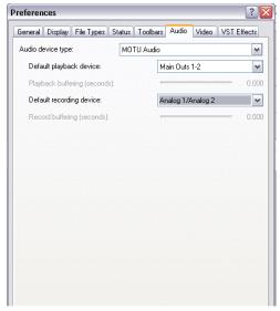
Figure 8-6: Enabling the 8pre driver in Sound Forge.
