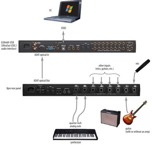
Figure 4-5: Using the 8pre as an optical converter.
