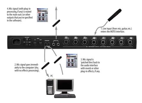
Figure 10-1: There are two ways to monitor live audio inputs with an 8pre: 1) through the computer or 2) via CueMix™DSP hardware monitoring. This diagram shows method 1 (through the computer). When using this method, use your host software's buffer setting to reduce the slight delay you hear when monitoring the live input, but don't lower it too much, or your computer might get sluggish.
