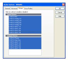
Figure 8-2: Activating the MOTU Audio WDM driver in SONAR by highlighting 8pre inputs and outputs.
