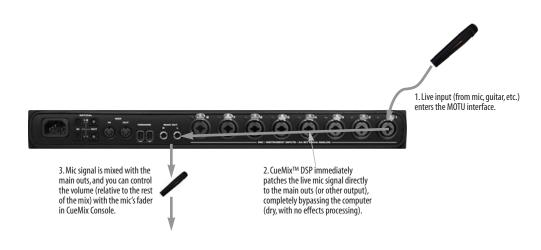
Figure 10-2: This diagram shows the signal flow when using CueMix $^{\text{TM}}$ DSP no-latency monitoring. Notice that this method does not allow you to process the live input with plug-ins in your audio software while it is being monitored. You can, however, add effects later — after recording the live input as a disk track. CueMix $^{\text{TM}}$ DSP lets you hear what you are recording with no delay and no computer-based effects.
