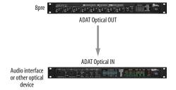
With this setup, in MOTU Audio Setup, choose the *Optical* clock source setting. The 8pre slaves to the optical device via their optical cable connection.
