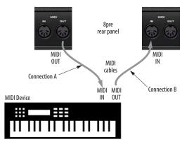
Figure 4-2: Connecting a MIDI device to the 8pre.
