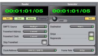
Figure 12-1: SMPTE Setup gives you access to your 8pre's on-board SMPTE time code synchronization features.
