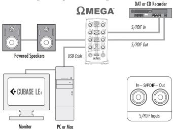
In this example we will show you how to record from a DAT player connected to the Omega Studio<sup>TM</sup> S/PDIF In directly into the software. Simply connect a 75 Ohm coaxial RCA cable from the DAT player's S/PDIF output to the Omega Studio's S/PDIF input.
