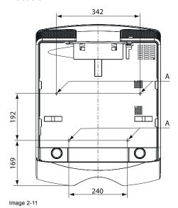
A: 4 mounting holes for ceiling mount plate. (M4, depth 10 mm)
