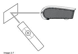
You can control the projector by the remote control signals reflected on the screen. However, the remote control distance may be restricted by the light reflection loss due to the screen characteristics.
