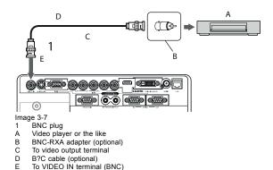
2. Connect the other end of the BNC cable to the video output terminal of the video equipment.
