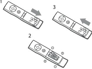
Image 2-5 Batteries insertion
