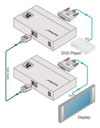
Figure 3: Connecting the 671T/671R Transmitter/Receiver System
