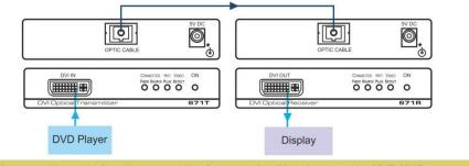
Always use Kramer high-performance cables for connecting AV equipment to the 671T, 671R.
