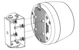
4. Attach the pivot plate assembly to the wall plate using the screw and washers previously removed. Tighten the screw.
