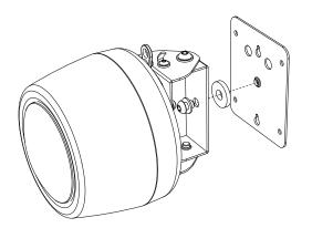
5. To adjust the position of the Stella-4, loosen the four pivot plate screws and position the Stella-4 as necessary. Tighten the pivot plate screws to secure the Stella-4.
