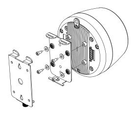
4. Attach the loudspeaker plate to the wall mount using the hinges and tighten the thumbscrew with a screwdriver (but don't over-tighten it).
