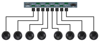
Figure 1: Stella-188 with Eight Stella-4s (One Unit Connected to Each Channel Output)
