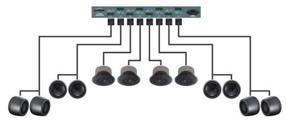
Figure 3: Stella-188 with Eight Stella-4s (Two Units Connected to Outputs 1, 2, 7, and 8) and Four Stella-8Cs (One Unit Connected to Outputs 3–6)
