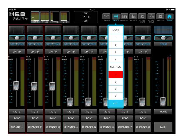
48V:Independently control 16 input channel's 48V phantom power on/off. Which channel requires 48V power supply, you lit the corresponding channel icon on.
