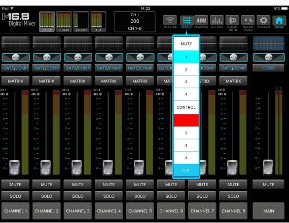
Control group: After entering control edit interface, as picture shows: after click "control 1", select 1,2,3,4 channel, and then select the simultaneous adjustment function that you want, then click control group"1", so that you can adjust the parameters of 1,2,3,4 channel at the same time.
