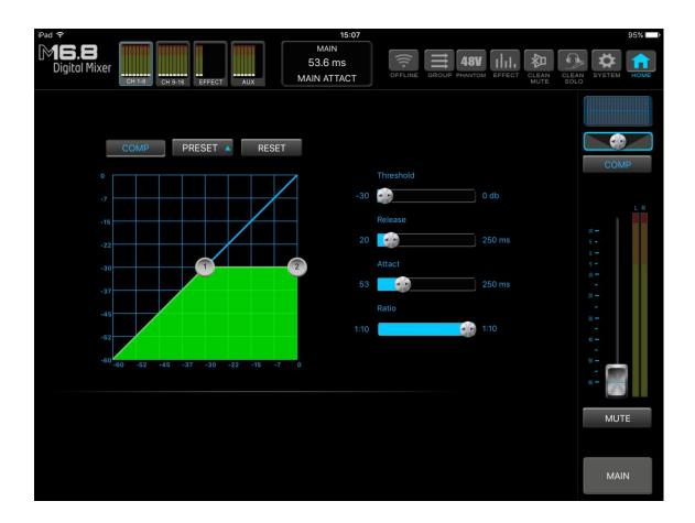
Threshold: Set the compressor threshold value (critical level),-60 dB~0 dB.
