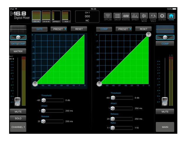
Compressor: It's a kind of amplifier with the input signal level increase and its own gain reduction.
