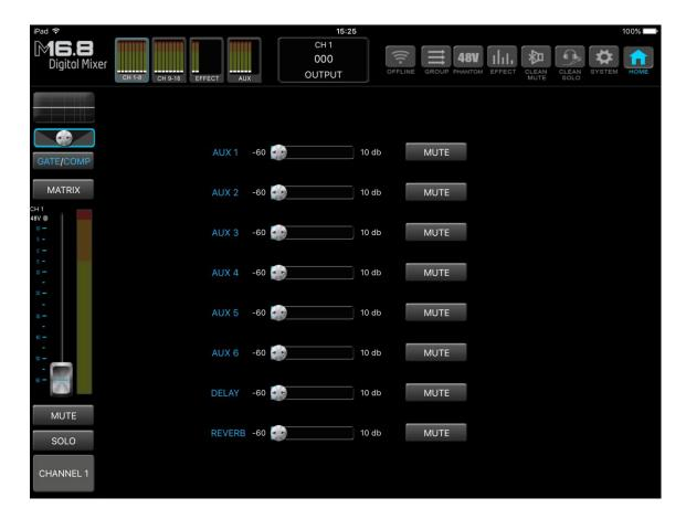
5.Input channel fader: Adjustable range -60 dB~10 dB.
