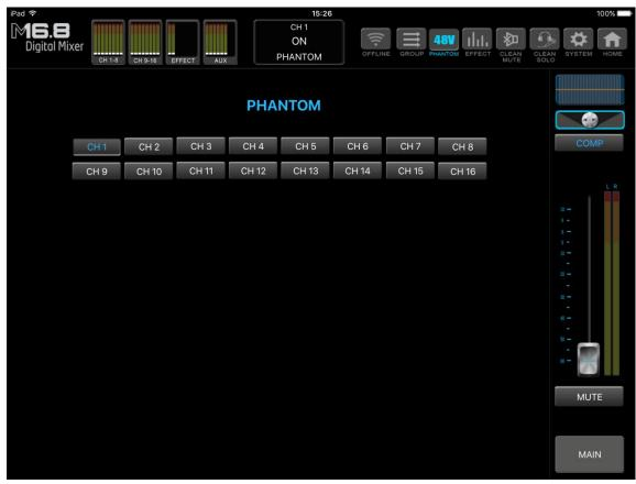
CLEAN MUTE: Click on this button, after 2 seconds, all channel mute function is deleted. CLEAN SOLO: Click on this button, after 2 seconds, all channel monitor function is deleted.
