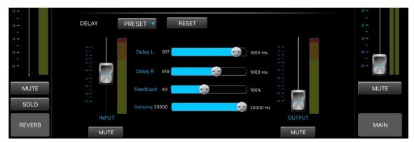
Delay Left: Control the interval time of the left channel echo, range is 10ms-1000ms.
