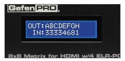
If all inputs are routed to their respective outputs, the front-panel display will appear as follows:
