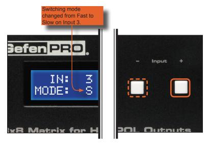
To change the switching mode of another input, press the **Output +** or **Output -** button to navigate to the desired input. Press the **Input +** or **Input -** button to toggle the switching mode between Fast (F) or Slow (S).
