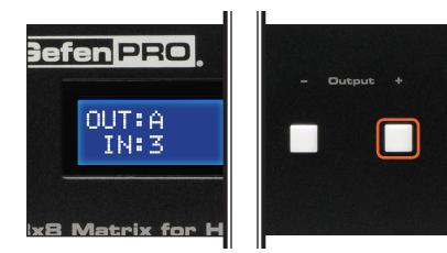
1. To select the output, press the **Out** - or **Out** + button once. The routing state for Output A will be displayed:
