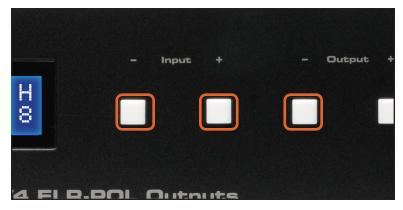
Use the Input + (or Input -) button to change the IR channel. Press the Input - button to decrease the IR channel value. Press the Input + button to increase the IR channel value.
