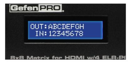
This is referred to as a "1-to-1" routing state. This is the factory (default) setting for the 8x8 Matrix for HDMI w/4 ELR-POL Outputs.
