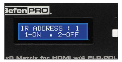
In this case, the 8x8 Matrix for HDMI w/4 ELR-POL Outputs is set to IR channel 1. Therefore, DIP switch 1 on the IR Remote Control must be set to the ON position and DIP switch 2 must be set to the OFF position.
