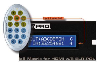
3. After the input and output have been selected on the IR Remote Control, the numbers on the far right-hand of the LCD display will disappear and the new routing state will be displayed in the LCD display:
