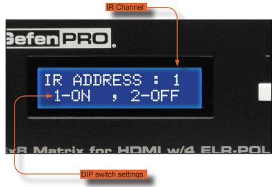
After setting the IR address, make sure that the DIP switches on the IR Remote Control are set according to the information in the LCD display. See page 11 for information on setting the IR channel for the IR Remote Control unit.
