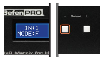
The letter **F** indicates that the HDMI input is using Fast Mode switching. If the HDMI input is set to Slow Mode switching, a letter **S** will be displayed under the input.  Press the Output - or Output + button again to cycle through the routing state for each output. Consecutively pressing the Output + button will cycle through each input, from left to right, starting with Input 1:
