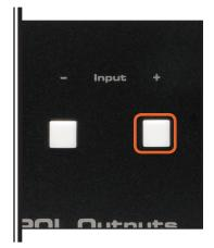
Consecutively pressing the Input - button will decrease the input value by a factor of 1 (within a range of 1 - 8). For example, if Input 3 was originally routed to Output D, pressing the Input - button will route Input 2 to Output D.
