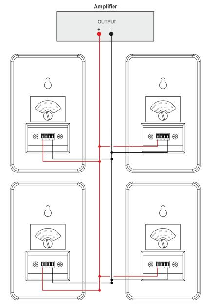
Figure 6 shows an example of parallel wiring in a square array installation:
