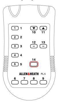
**Labelling the buttons** If required, the installer can adhere a custom label to the controller surface. We advise that this is made using a strong, waterproof and dirt resistant material. For reference the top to bottom dimension of the keypad area is 60mm.
