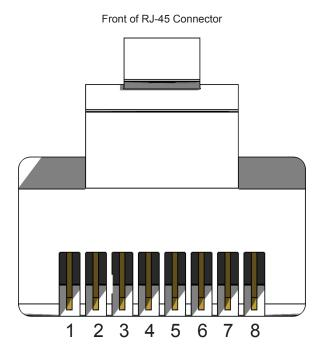
Gefen recommends the TIA/EIA-568-B wiring option. Use the table below when field-terminating cable for use with Gefen products.
