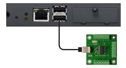
Connect open-close switches to the 10 Input ports and connect low-current (max. 50mA total) lights and actuators to the 4 Output ports. Refer to the schematic below.
