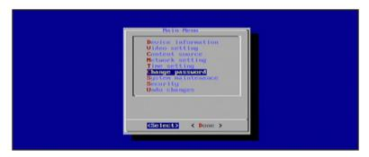
Enter the password under the Change Password dialog. If no password was previously set (or if the unit has been reset), then the Old Password field will be blank. Use the ▲ and ▼ keys to move between each field.
