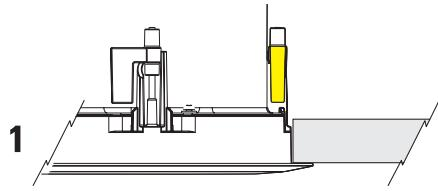
After the cabinet is installed into the mounting cutout, tighten each clamp's screw using a #2 Phillips screwdriver, see 2, right.
