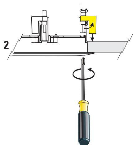
The clamp rotates 90° and is then pulled tight by the screw, see 3, right.
