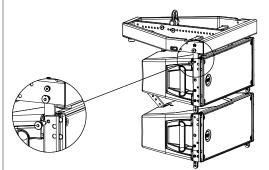
4) Reverse and connect the 1 rear bracket to the fly-bar using 2 quick lock pins. The first HDL has to be fixed always starting at 0° with respect of the frame. No other angles are allowded.
