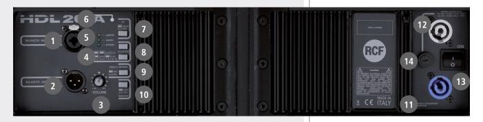
MAIN XLR INPUT (BAL/UNBAL). The system accept male XLR/Jack input connectors with line level signals from a mixing console or other signal source.
