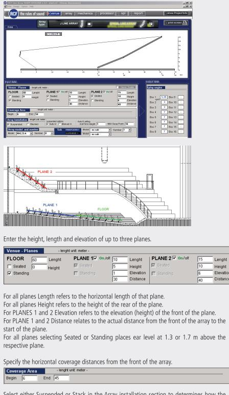
Select either Suspended or Stack in the Array installation section to determines how the array is supported.  $\ensuremath{\mathsf{S}}$
