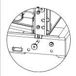
2) The stacking bar adds a fixed amount of up or downtilt to ground-stacked HDL loudspeakers, with additional 15 degrees of adjustment possible (from  $+7,5^{\circ}$  to  $-7,5^{\circ}$ ).
