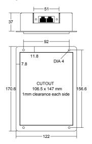
**Connecting to PL-Anet** PL-Anet is the proprietary Allen & Heath system for daisy chaining PL remote controllers. It is an RS485 serial connection that uses CAT5 STP cable to communicate between devices over long distances. The connection includes +20V DC to power the connected devices. Use flame retardent CAT5 STP (shielded twisted pair) RJ45 cables. The **iDR-8** main unit port is shown here.
