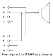
IN speakON<sup>®</sup> point 2-1+ 2+ 1-LF + LF -NC NC Connection  $\square$ 0 0 nar MODEL: IBZA6HZ POWER: MPEDANCE: 40 OHM 180101/001 SERIAL N:
