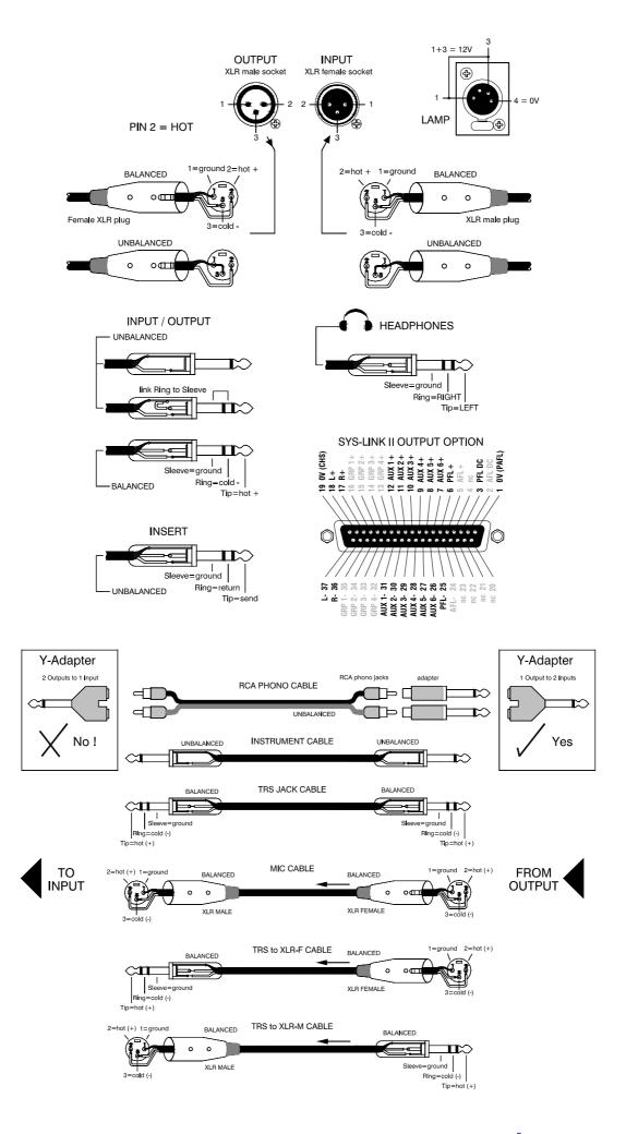
The MixWizard uses professional grade 3 pin XLR and 1/4" TRS (3 pole) jack sockets. To ensure best performance, we recommend that you use high quality audio cables and connectors, and take time to check for reliable and accurate cable assembly. It is well known that most audio system problems are due to faulty or sub standard interconnecting leads. The following mating plugs may be used to connect audio signals to the console:
