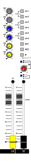
**AUX MASTERS** Each aux mix has a master level control that adjusts the output level to match external equipment, or to trim the monitor, effect or other send without affecting the mix balance. Up to +4dB boost is available above the normal 0dB position.
