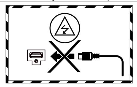
Prior to connecting any device to this unit, switch the projector in standby mode. Never connect a HDMI source to this unit when the projector is in operate mode. The HDMI termination is a self-powered connection and can cause electric discharges.
