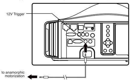
Connect the lens motorization to the 12V Trigger output
