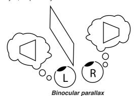
3D movies use two sets of images: one set for the left eye, the other set for the right eye. These images can be stored into three compatible formats: Frame packing, Top-&-Bottom or Side-by-Side.
