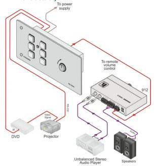
Figure 3: Connecting the RC-52A
