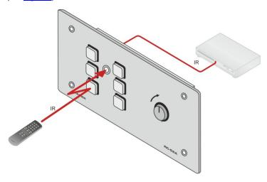
Figure 7: IR Repeater Operation
