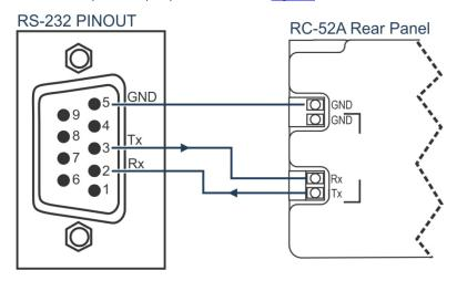
Figure 4: RS-232 Pinout
