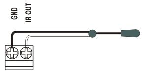
Figure 6: IR Emitter Wiring
