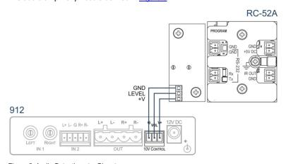
Figure 5: Audio Potentiometer Pinout
