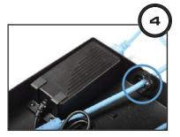
Run all connector cables out through the back of the unit. Use the included split grommets to protect the cables, as shown in the photo below:
