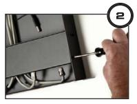
Use a Phillips screwdriver and disconnect the clamping plate by removing the two (2) screws on each side of the Rack Tray.
