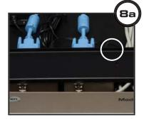
**IMPORTANT:** When reassembling the clamping plate, make sure that the raised lip on the top of the clamping plate faces the back of the Rack Tray.
