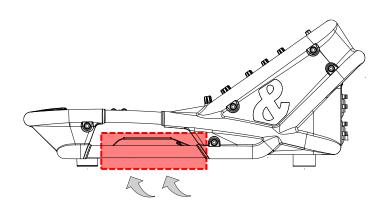
Leave adequate space for (1) ventilation (\*) and (2) USB / headphone connections at front of mixer.
