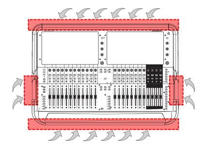
Leave adequate space for ventilation (\*) at the sides of the mixer in the area indicated.
