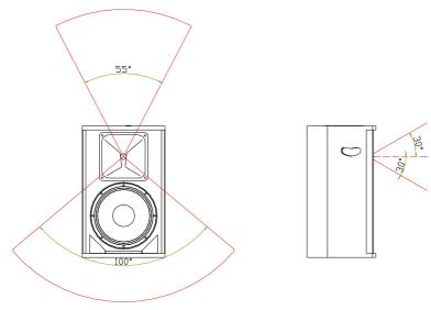
The horn of V-10 loudspeaker is mounted at the factory in such a way that the horizontal coverage is  $90^{\circ}$  and the vertical coverage is  $60^{\circ}$ . You can easily re-orient the V-10 rotatable horn to its  $60^{\circ} \times 90^{\circ}$ .
