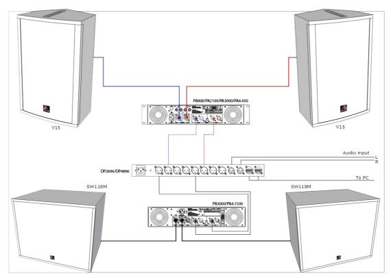
Fig.9.- 1 x V-15 + SW-118M L/R configuration
