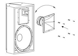
Fig.3.- Change of configuration on V-10
