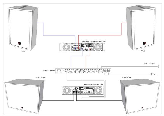
Fig.7.- 1 x V-12 + SW-118M L/R configuration
