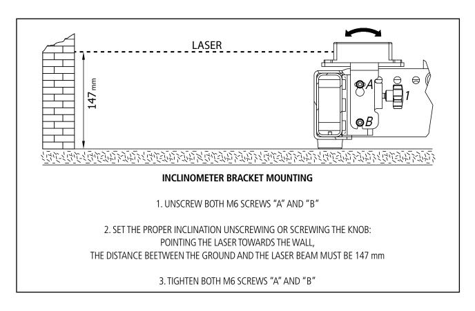
Note that using Rd-Net to set up the system, there will be the possibility to monitor the angles of the flybar and of each single speaker and in case using 1 pick-up point, appropriately calculated by RCF Easy Shape Designer, the cluster will take the proper aim and angles without the need of the inclinometer.
