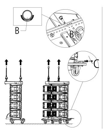
Begin to lift the flybar, and when it goes on traction on the first module, insert the locking pin in the hole "B".
