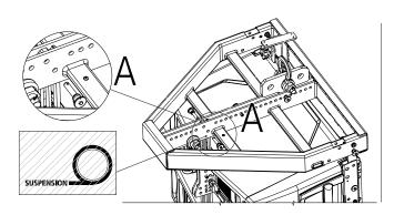
Lift up the rear bracket of the highest cabinet. Insert the quick lock pin in the "suspension" hole "A" of the flybar.
