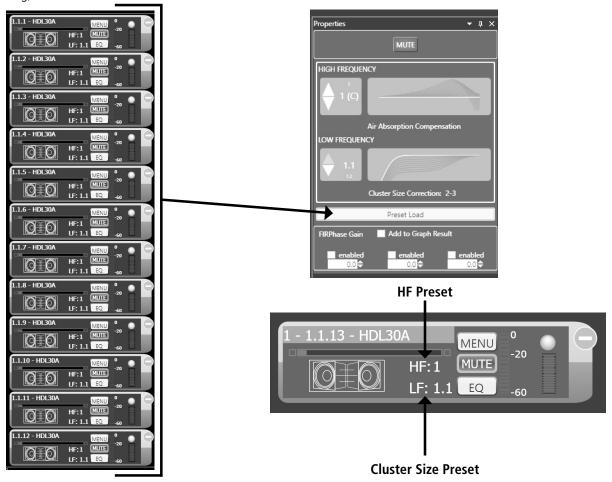
As descripted for the Low Frequencies, the user may need to scala up or down the presets set maintaining the compensation ratio between all the cabinets. This scaling operation can be performed with the arrow button in the group tab. Even though the presets change is possible on every single loudspeaker, a global change by using the group properties tab is strongly recommended in order to preserve the air absorption compensation distribution all along the audience.
