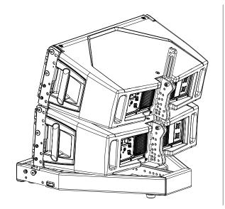
Fix the next module with the front quick lock pins. Lift the rear part of the module, insert the locking pin in the proper position and release the module leaning with the right angle.
