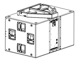
Fix the flybar to the stacking kit using the two quick lock pins.
