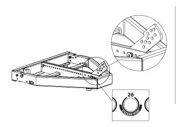
Fix the stacking bracket in the hole number 26 of the flybar and orientate it as shown in fig 2.
