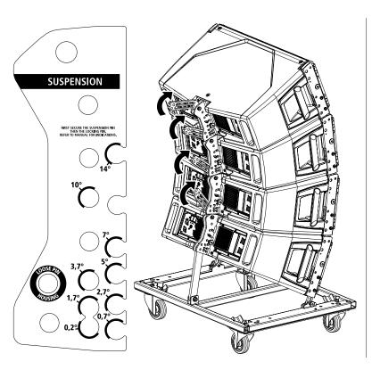
Hook the flybar to the chain and lift the flybar to a suitable height for the first cabinet.
