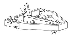
A maximum of 4 x TOP cabinets are allowed to be set up as ground stack.
