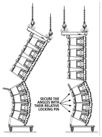
Pull out the front and rear pin from the cart and remove it
