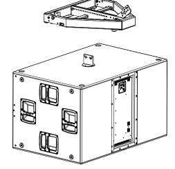
Place the flybar to sub and insert the stacking kit between the two cental pipes.
