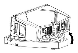
Turn the rear stacking bracket of the flybar and select the proper angle. The correspondence of the bracket's holes is the following:
