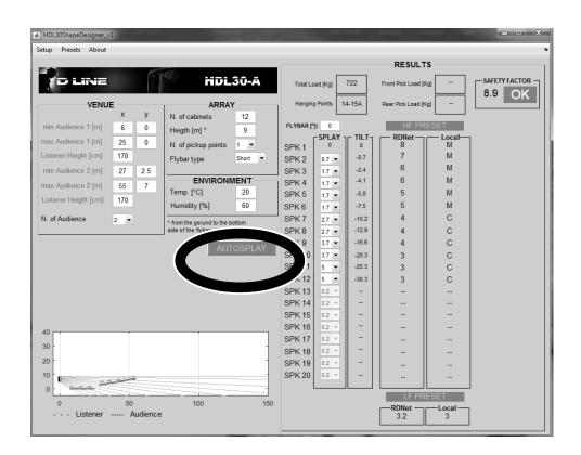
Every time the user changes flybar tilt, splay angles, humidity, temperature or height of the array, the software automatically recalculates the presets. It is possible to save and load a project of the Shape Designer using the "Setup" menu.
