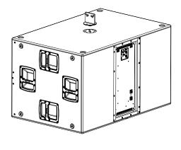
On subwoofers 8006, 9006 and 9007 series fix the optional accessory "STACKING KIT STCK-KIT 2X HDL 30" cod. 13360393, to M20 female screw on the upper part of the sub.
