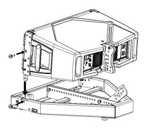
Place the first module fixing the front bracket into the fixing point "A" of the flybar using the quick lock pins of the flybar.
