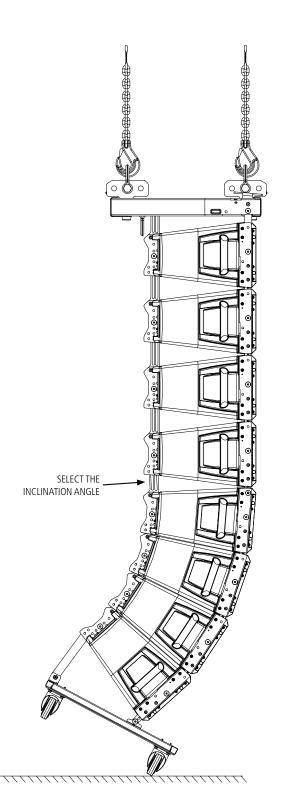
Working with one pick up point this is achieved by pushing forward the cluster and simultaneously lowers the height of the system.
