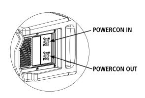
Each HDL 30-A module is provided with a Powercon outlet to daisy chain other modules. The maximum number of modules that is possible to daisy chain is:
