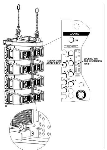
Stop lifting and insert and lock the second Locking pins (Safety pins) to prevent the system from going into compression shifting the tilt of the module, and consequently of the cluster.
