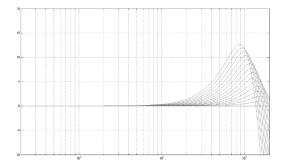
A low pass filter is progressively introduced with the increase of the compensation gain: the system does not need to reproduce frequencies that could hardly reach the desired distance and that could lead to a waste of useful energy. The picture below (Figure 6) shows the behavior of the 15 filters. These filters are designed as very small FIR (finite impulse response) filters in order to preserve the phase coherence of the system.
