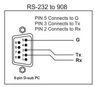
Figure 7: Connecting to a PC
