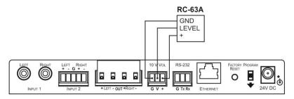
Figure 6: Connecting the 10V VOL Terminal Block Connector
