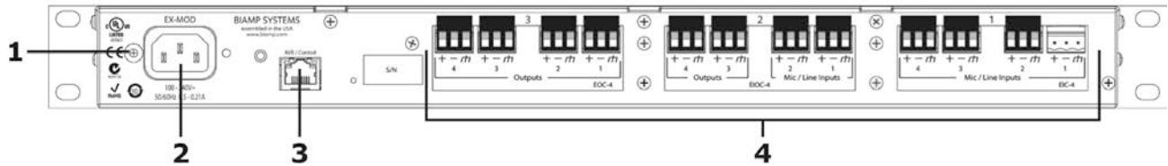
**1. Grounding pin.** This pin is for grounding the chassis of the expander.
