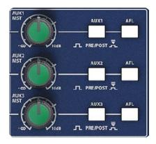
The Aux Master Output channel determines the output level of a whole Aux mix (the sum of all Aux contributions). That is, the Aux 1 Master controls the Aux 1 output level, which is the sum of all Aux 1 contributions from the input channels.
