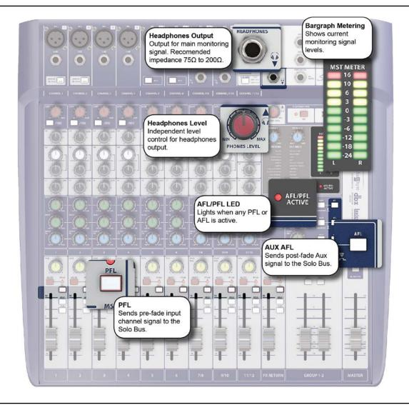
The Signature's Solo and monitoring system allows an engineer to hear either the Master (MST) stereo outputs or any channels currently assigned to the Solo bus, via the headphone output.
