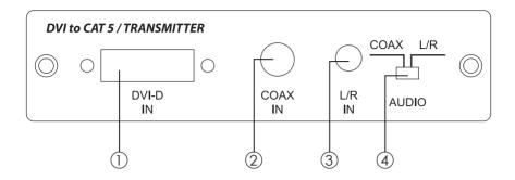
DVI-D IN – Plug from DVI/HDMI source equipment's video output with DVI in cable.
