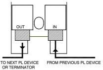
End of chain termination As with any RS485 system, the last PL device needs to have a terminating resistor fitted to its output port. Early version PL-3 modules are shipped with a 100 ohm resistor already fitted. Leave this fitted only if the unit is the last in the chain. Later version PL-3 modules are supplied with a terminating RJ45 plug (Allen & Heath part number 003-082).
