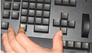
If the lifting – device is used intensively, it can happen, that the motor ist temporary switched off by the temperature control. During that period adjust the monitor-wing manually: press and hold **MA** and **Set** – button und adjust the wing. After releasing the buttons this position is fixed.
