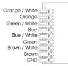
Figure 4: WP-306 Wall Plate EU/UK TP Terminal Block Pinouts
