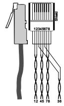
Figure 2: RJ-45 Pinout (U.S.)
