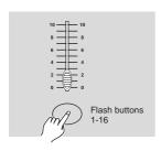
Tap the Flash button numbered from 1-16 to assign MIDI IN channel 1-16, the relevant channel LED lights indicating MIDI IN channel is set.
