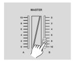
3. Push Master Slider B to its maximum position(fully down).
