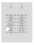
Create a desired scene using Channel Sliders 1-24. At 0% or DMX 0, these sliders should be at 0 position, and at 100% or DMX 255, these sliders should be at 10 position.
