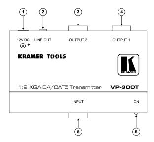
Figure 4: VP-300T 1:2 XGA DA/ CAT 5 Transmitter (Topside)
