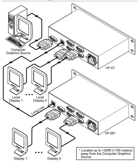
Figure 12: Connecting the VP-5T and the VP-5R
