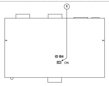
Figure 5: VP-300T 1:2 XGA DA/ CAT 5 Transmitter (Underside)
