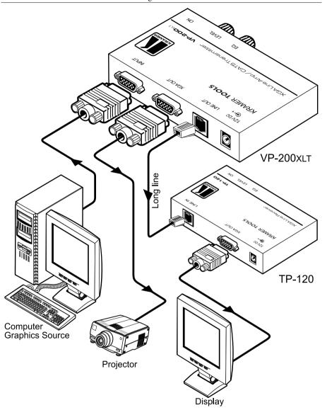
Figure 10: Connecting the VP-200XLT
