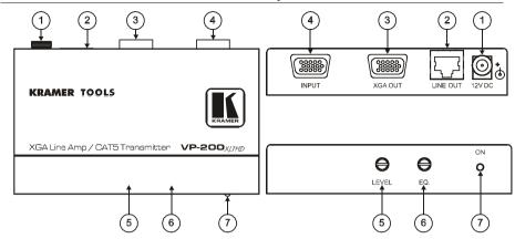
Figure 2: VP-200XLTHD XGA Line Amp / CAT 5 Transmitter
