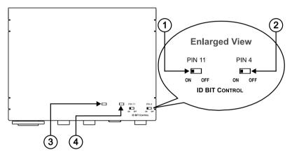
Figure 7: VP-5T/VP-5THD 1:4 VGA/UXGA Distributor / CAT 5 Transmitter (Underside)
