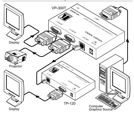
Figure 11: Connecting the VP-300T
